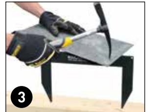
3 TO PUNCH HOLES PLACE TILE WITH MARK JUST OVER EDGE
